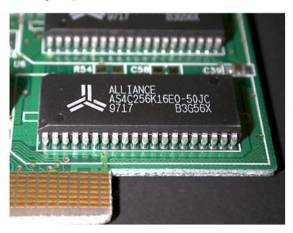
b. Squeeze a small amount of non-corrosive silicone onto a clean piece of paper. Use the small end of the Arctic Silver mixing wand to cover the chip leads with silicone. Wipe the mixing wand thoroughly to remove all the silicone.
