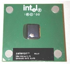
Put the dab of Arctic Silver II you removed from the heatsink base onto one corner of the CPU core as shown in the photo to the left.
