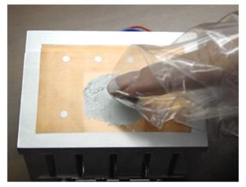
Tint (stain) the bottom of the heatsink in the area where the CPU core will contact it. Put a finger into a plastic bag and thoroughly rub the compound into the base of the heatsink using both clockwise and counter-clockwise circular motion as shown in the photo to the left. This will ensure optimum filling of the microscopic valleys in the metal.
