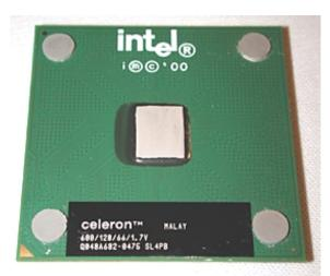
Spread the Arctic Silver II over the CPU core as shown in the photo to the left. The small amount transferred from the heatsink in the step at the top of the previous page has been carefully spread over the top of the core using a single edge razor blade. A razor blade or the clean edge of a credit card can be used as the application tool. You may use whatever tool you choose as long as it is CLEAN and allows you to control the application area and thickness.
