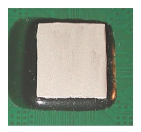
RECHECK to make sure no foreign contaminants are present on either the bottom of the heatsink or the top of the CPU core. Mount the heatsink on the CPU in the proper orientation per the heatsink's instructions. Verify that the pressure point on the clip is directly above the CPU core.
