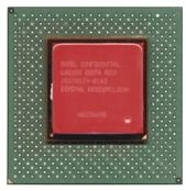
Note that on the Intel P4, the compound is applied to the integral heat spreader. (The metal cap that covers the actual CPU core.)
