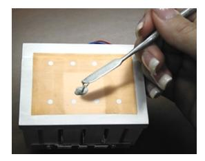
Using a clean razor, the clean edge of a credit card, a clean knife, or some other appropriate clean tool, pick up a small dab of the Arctic Silver compound from the mound you put on the heatsink as shown in the photo above on the right.
